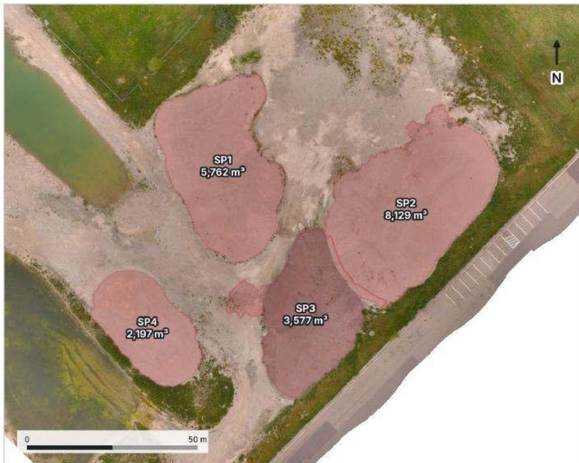
Figure 6.1 · Stockpile footprints and measured volumes
