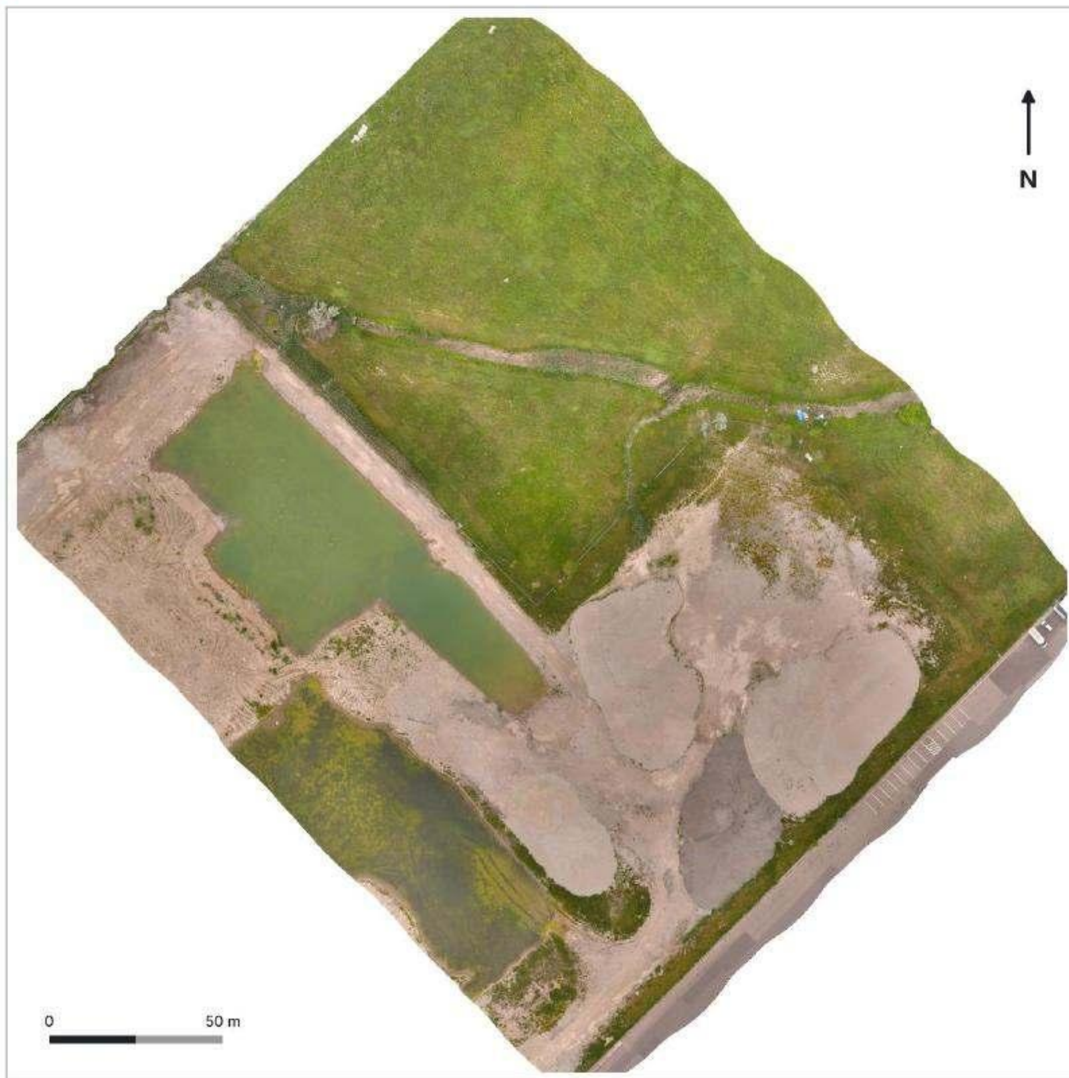
Figure 3.1 - True orthomosaic, 3 cm ground pixel, 5.8 ha.
