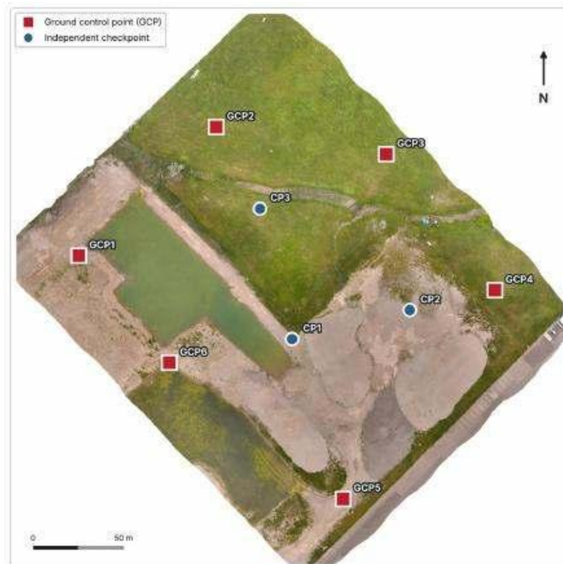
Figure 9.1 · Recommended ground control (6) and checkpoint (3) layout for the next visit:
